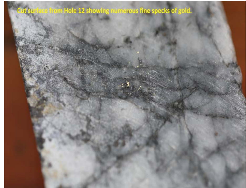
Core showing closeup of gold from DDH 21-12.
