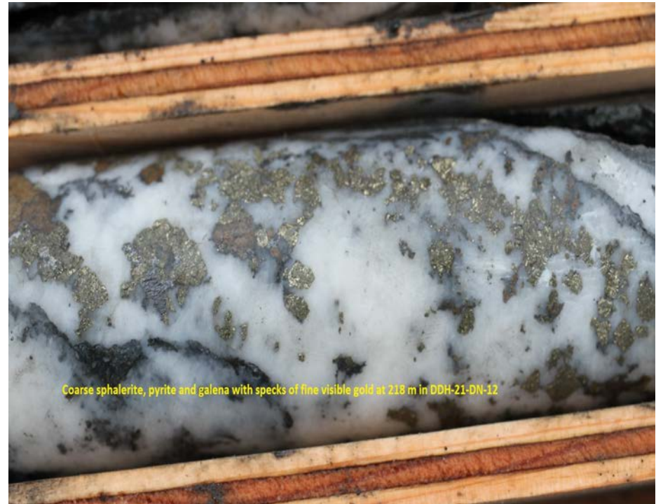
Core from DDH 21-12 showing sphalerite and galena.
