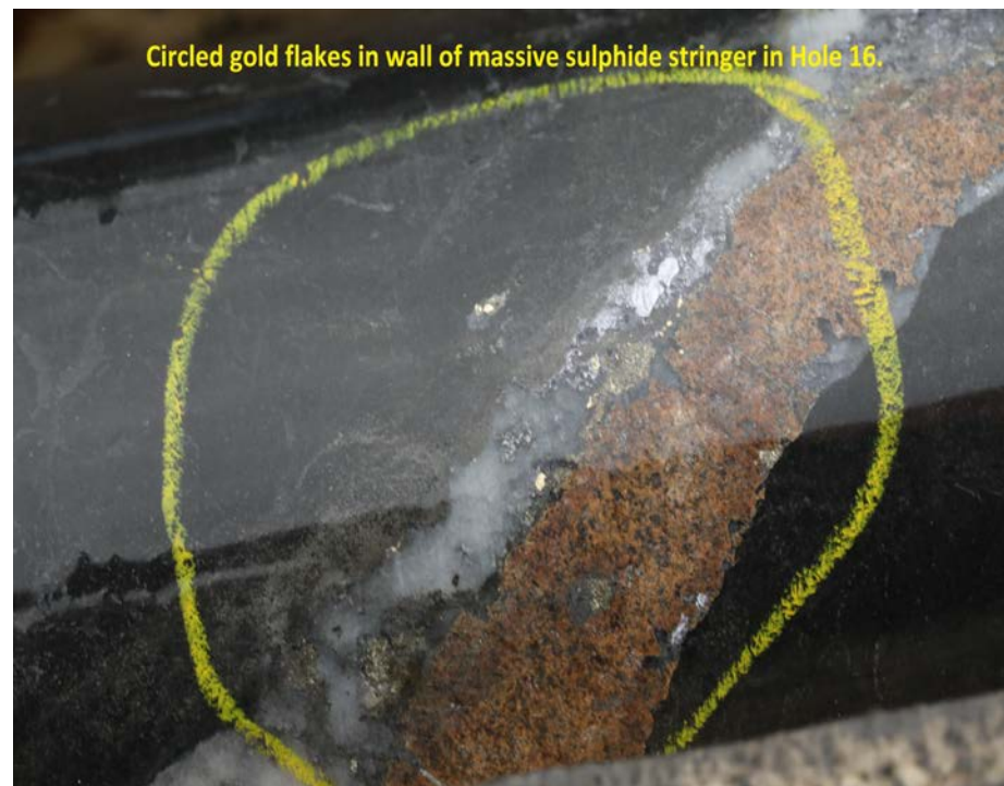
Section from DDH 21-16 showing 3.96m of 1.51 g/t Au and 167 g/t Ag.
