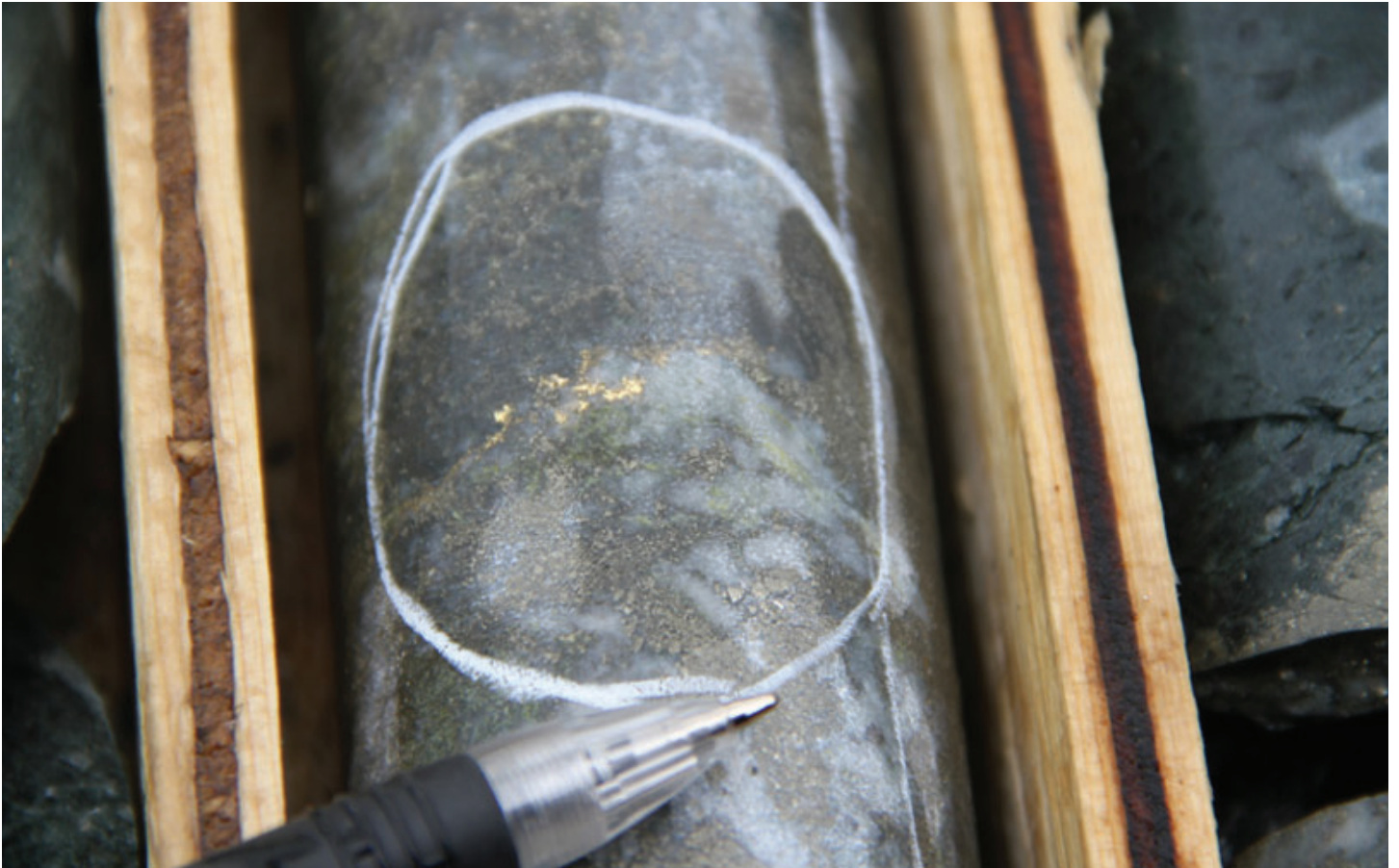
Photo showing visible gold in 2010-DDH-RC-5 from the Red Cliff zone.
