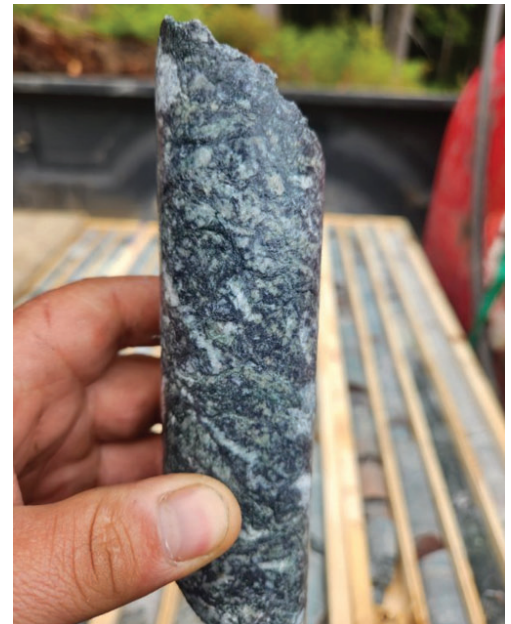
Photo shows semi-massive pyrite and arsenopyrite in sample 24-JN-3.
