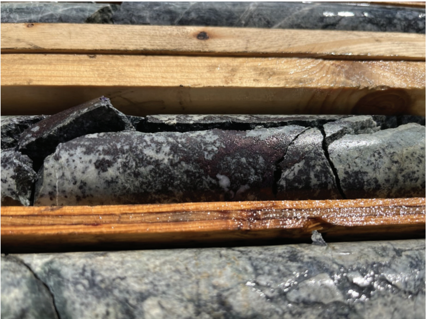
Above photo showing coarse bornite in DDH-NB-24-13
