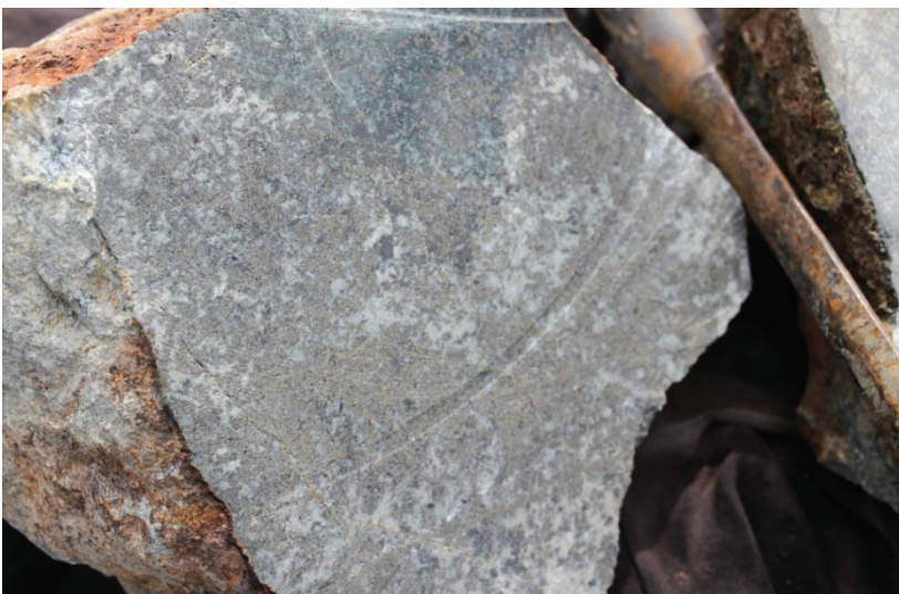
Photo shows semi-massive pyrite and arsenopyrite in sample 24-JN-3.
