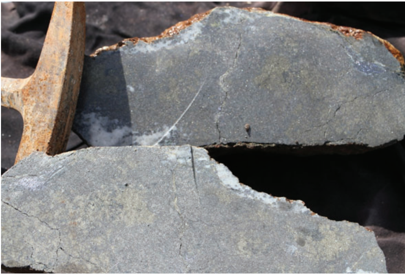
Photo shows massive sphalerite, pyrite and arsenopyrite in sample 24-JN-5.
