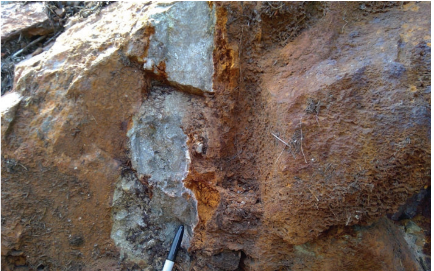
Photo showing semi-massive pyrite and chalcopyrite above the Red Cliff adits.
