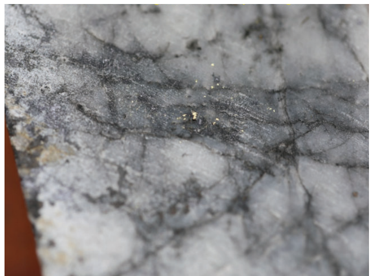
Cut surface from Hole 12 showing numerous fine specks of gold.
